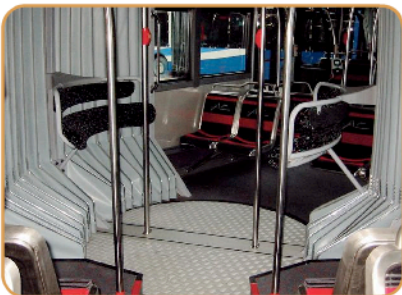
Van Hool easy walk through turn table is usable while bus is in operation
